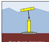
Wave Energy Converter Seabed-based buoy
