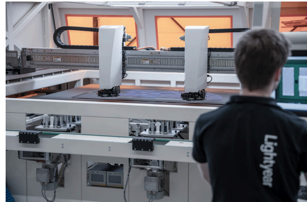
Manufacturing of a Lightyear VIPV panel in the Netherlands.
